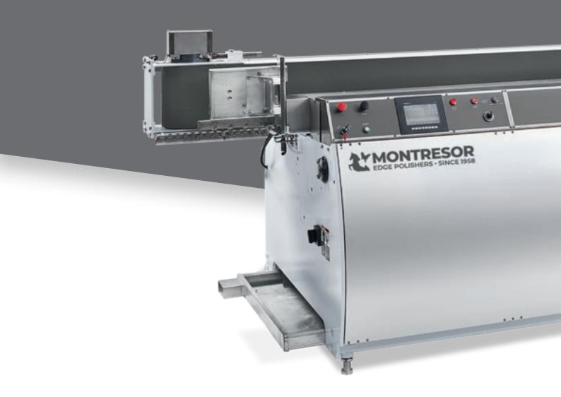
**Vela 7.2** is the compact, innovative vertical edge polisher that can polish flat edges of granite, quartz, ceramic and marble from 10 to 60 mm in thickness.
