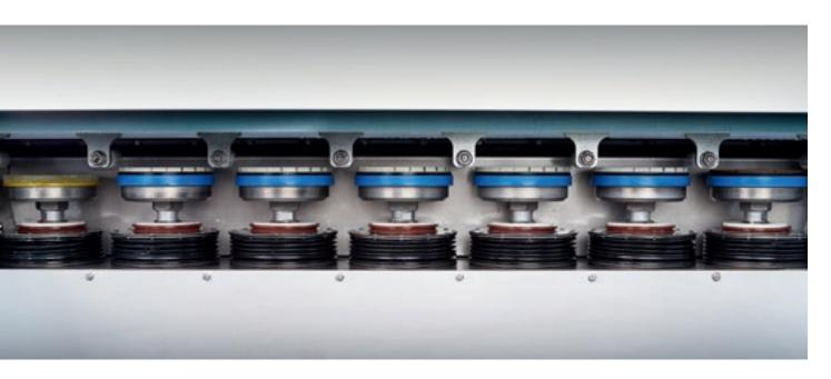
Vela is equipped with 7 micro-oscillating frontal units, providing excellent results even in the event of slight cutting defects or edges that are not perfectly aligned
