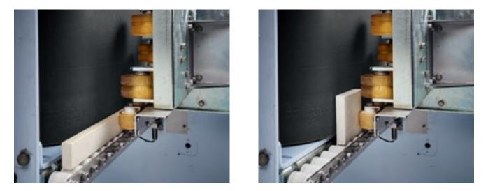
Innovative system with double conveyor belt to guarantee perfect stability, even when working with narrow pieces from 45 mm and heads from 60 mm.
