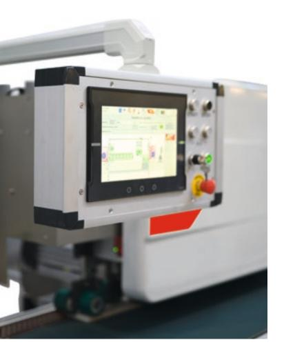
Control panel with swivel arm enables work from different angles and provides maximum visibility and ergonomics for the operator.
