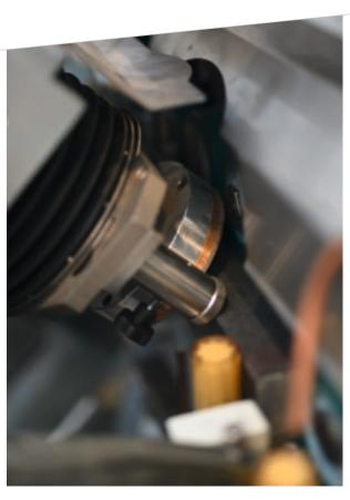
Creation of chamfers of a consistent size courtesy of the upper chamfering unit which "adapts" to the thickness of the material, with an automatic and manual slide block system.
