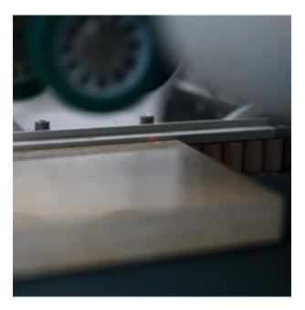
Automatic reading of the thickness of the panel for automatic adjustment of the devices.
